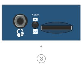
Figure 2-4: Monitoring facility and SD-Card slot
